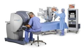
The surgical cart utilises one robotic arm to control the endoscopic camera which provides 3D vision, and three robotic arms to control surgical instruments. It is located next to the patient and allows the ability to rotate the instruments with unrivalled precision and control, using only a few small incisions.
